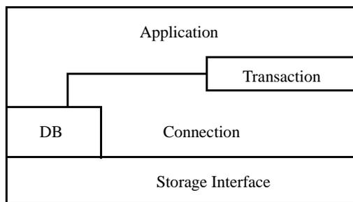
**Figure 2.** Layered view of the ZODB architecture
