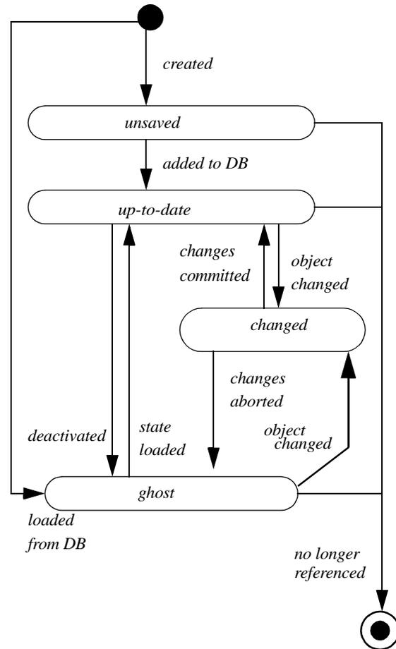
Figure 1. State diagram showing in-memory persistent object states and transitions.
